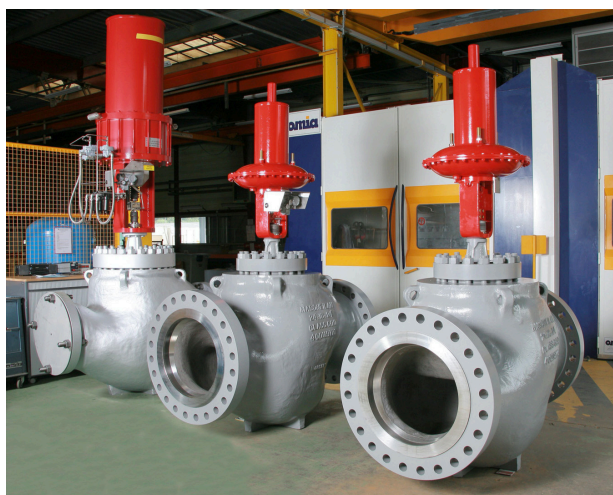
Figure 3. Large inlet gas globe control valves, Masoneilan 41005 series.
