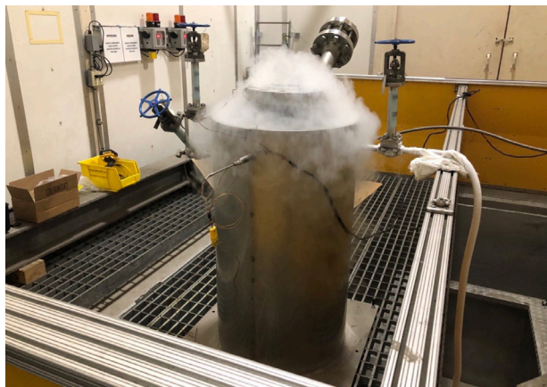
Figure 1. A cryogenic test rig for relief valves.
