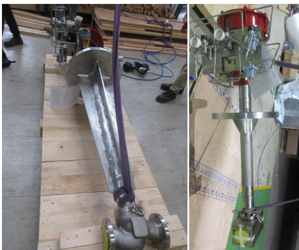
Figure 5. Globes with elongated and re-inforced bonnets, and bellows ring for cold box.
